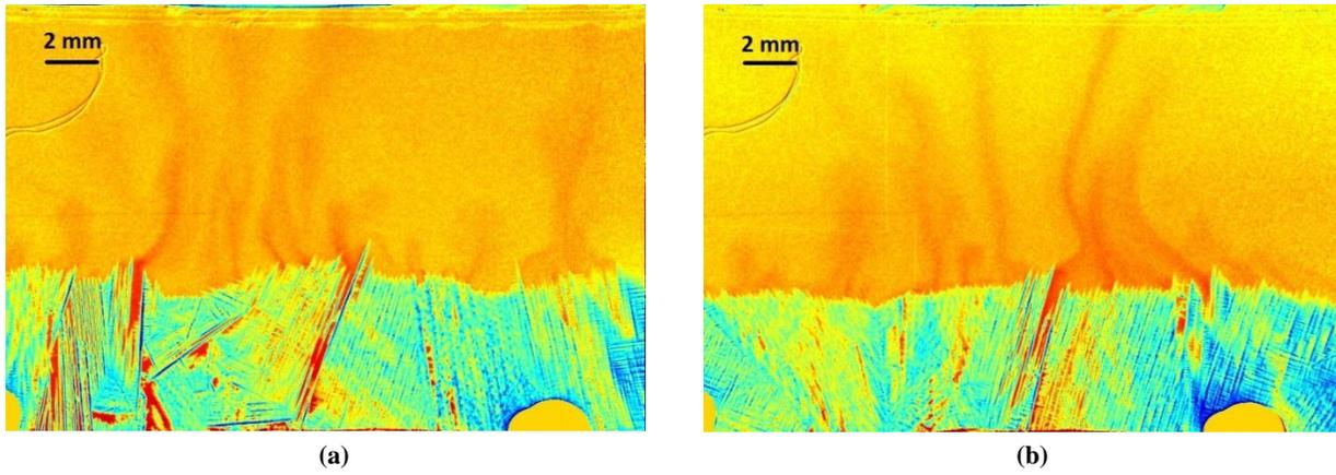
Figure 6: Snapshots of dendritic structure and composition field obtained from two solidification experiments at a cooling rate  $R = -0.01 \text{ K s}^{-1}$  and temperature gradients of (a)  $G = 1.1 \text{ K mm}^{-1}$  and (b)  $G = 1.3 \text{ K mm}^{-1}$
