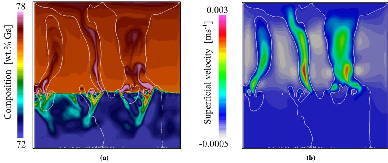
**Figure 9: Results for case CAFE\_G1R2L1 at 350 s showing (a) the average gallium composition and (b) the vertical component of the superficial velocity. The white contour identifies the zero velocity limit for the vertical component of the superficial velocity field.**
