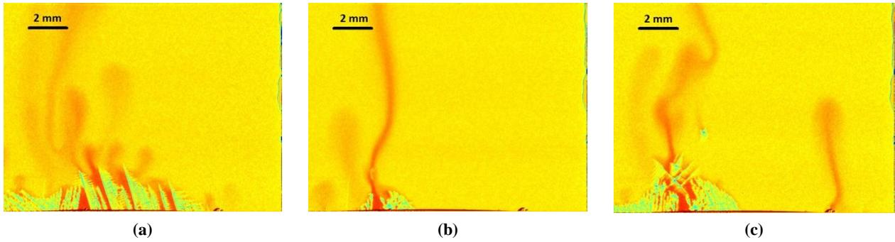
**Figure 8: Snapshots of dendrite structure and composition field from two solidification experiments conducted at a cooling rate  $R = -0.01 \text{ K s}^{-1}$  and a temperature gradient  $G = 1 \text{ K mm}^{-1}$ : (a) “pulsing” plumes, (b) continuous plume, (c) upcoming instability of the plume**
