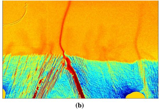
**Figure 1: Illustration of the benchmark experiments for in-situ observation of segregated channels using X-Ray radiography with (a) a schematic of the cell and (b) a typical image of the microstructure formed during directional solidification of an In - 75 wt.% Ga alloy [2]**
