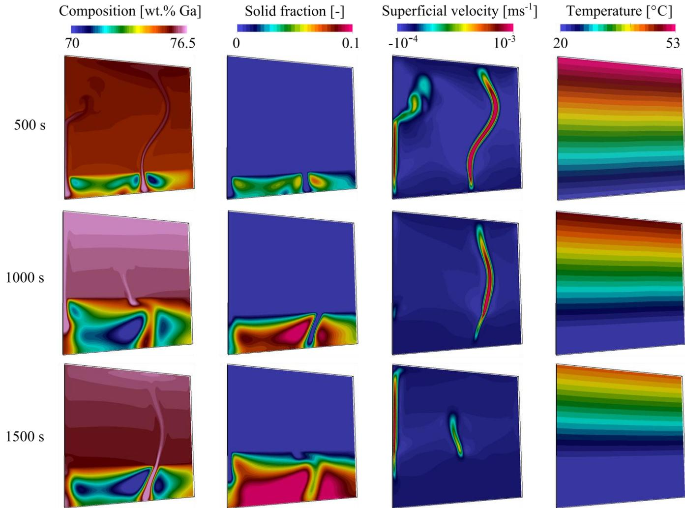
Figure 4: Simulation results for case FE\_G2R1L1 showing, from left to right, maps of the average Ga composition, the solid fraction, the vertical component of the superficial velocity field and the temperature on a cut plane at the center of the cell at 500 s, 1000 s and 1500 s.
