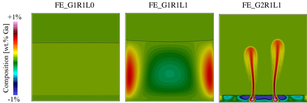
**Figure 3: Average composition field at 250 s for the 3 FE cases showing the influence of the process parameters on the tendency to form channel segregation and convective plumes. The black line represents the liquidus isotherm given in Table 1.**
