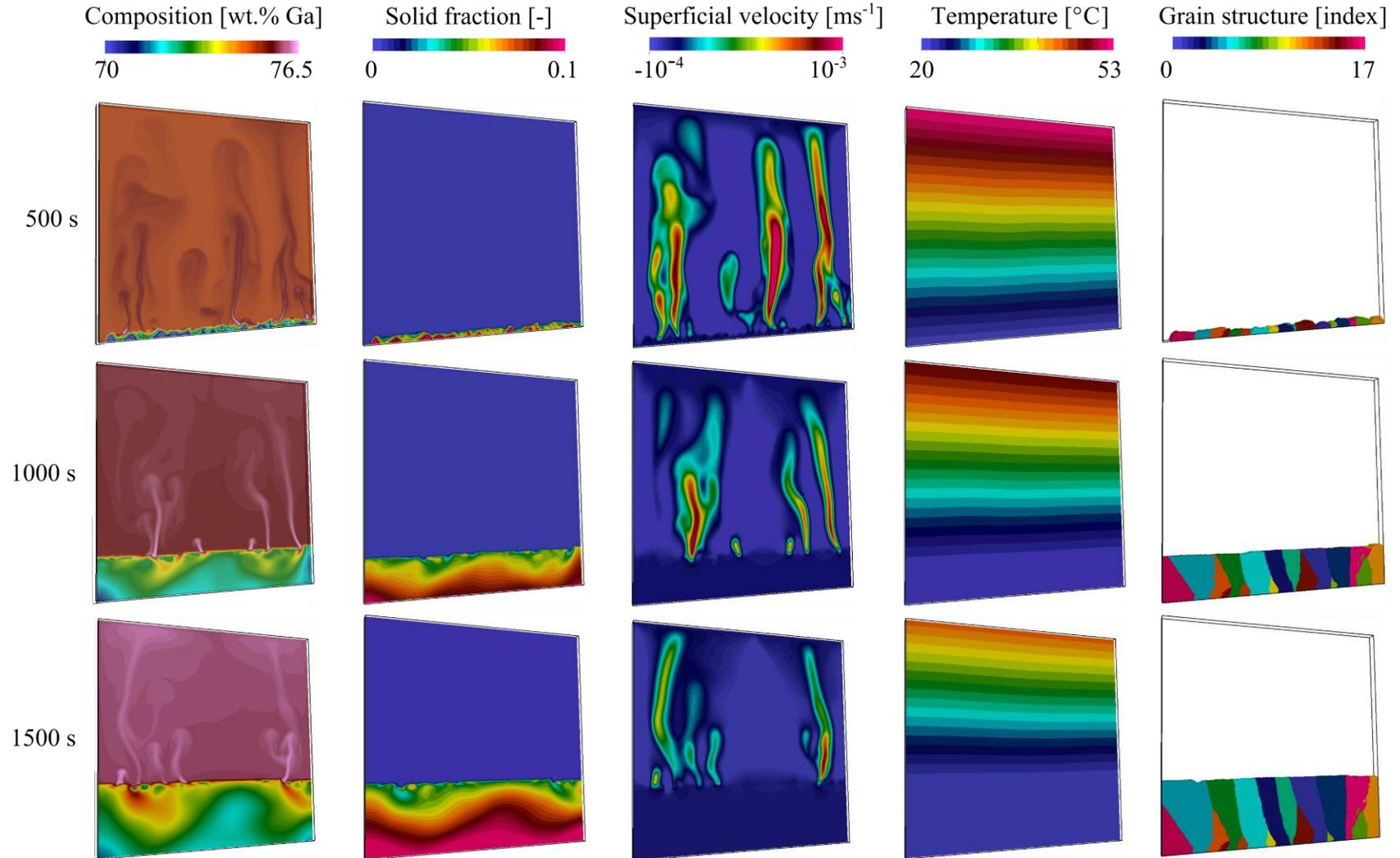
Figure 5: Results for CAFE\_G2R1L1 case showing average composition, solid fraction, vertical component of the superficial velocity and temperature while the last column shows the grain envelopes predicted by the CAFE model.
