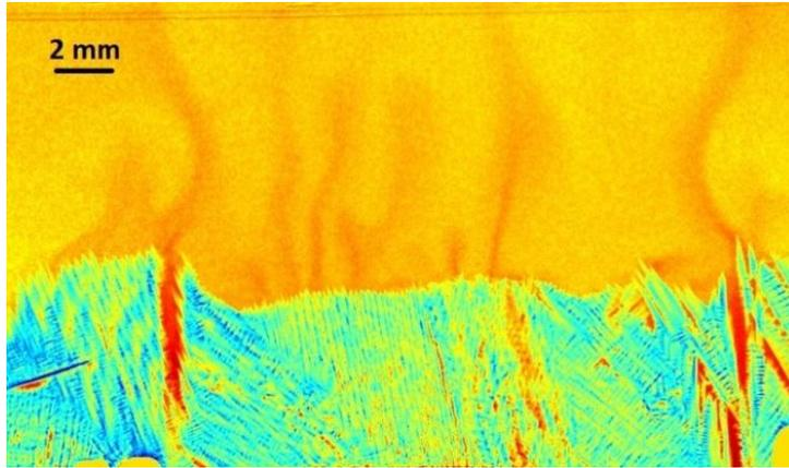
Figure 11: Snapshot of dendritic structure and composition field from a solidification experiment recorded at 1000 s for a cooling rate  $R = -0.01 \text{ K s}^{-1}$  and a temperature gradient  $G = 1 \text{ K mm}^{-1}$
