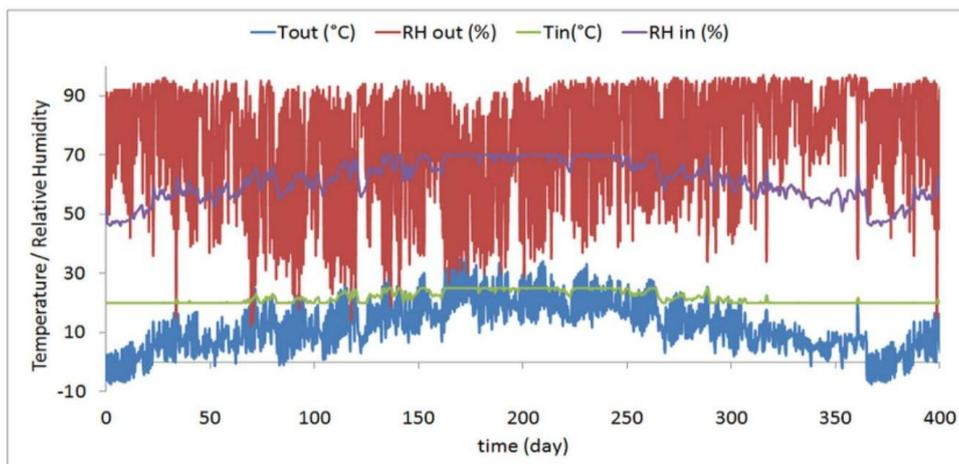
Figure 3: Exterior and interior air temperature and relative humidity over one year for Grenoble
