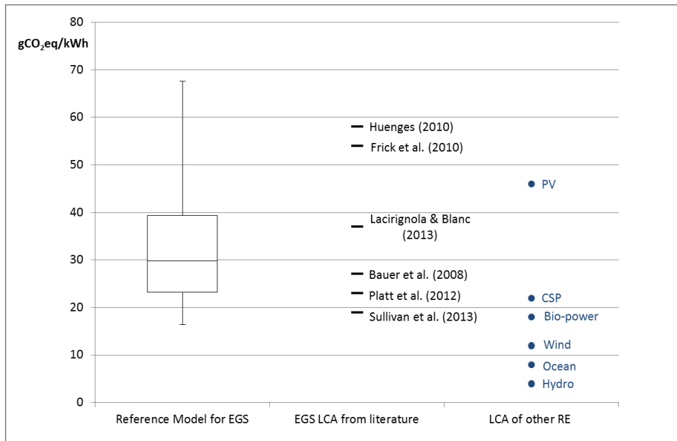
Figure 2: Results of the reference model (GHG profile) compared with LCA results from literature regarding EGS and other renewable energy technologies. Whiskers indicate the 5 th and 95 th percentiles. The box indicates the 25 th and 75 th percentiles.
