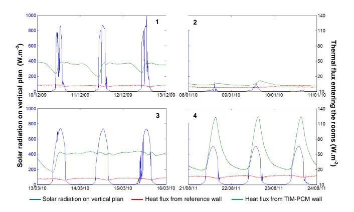
Fig. 7. Heat gains through the reference and the TIM-PCM walls and solar radiation for the four specific climate conditions
