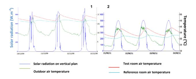
Fig. 8. Solar radiation and air temperatures for three days in December and August
