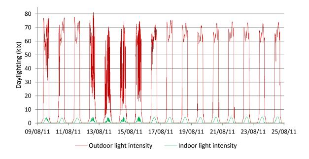
Fig. 10. Measurements of the daylighting outdoor and within the test room for 16 days in December and August
