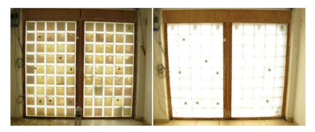
Fig. 9. Daylight provided by the TIM-PCM wall with the PCM in solid state (left) and liquid state (right). The picture is taken from inside the test room
