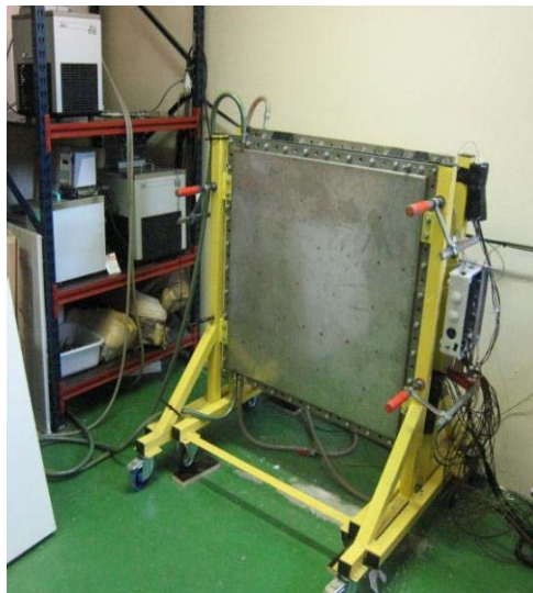
Fig. 4. Small size prototype within the double heat exchanger test rig
