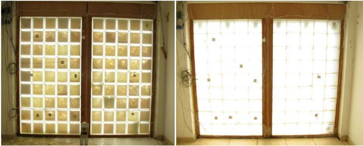
Fig. 9. Daylight provided by the TIM-PCM wall with the PCM in solid state (left) and liquid state (right). The picture is taken from inside the test room
