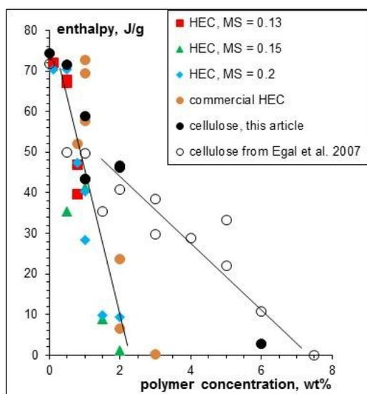
Fig 3 - Enthalpy of the eutectic peak as a function of polymer concentration for cellulose and the four HEC samples in 8%NaOH-water.
