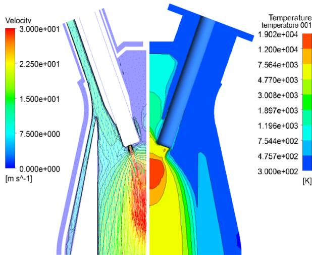
**Figure 7.** Velocity field (left), temperature field (right).
