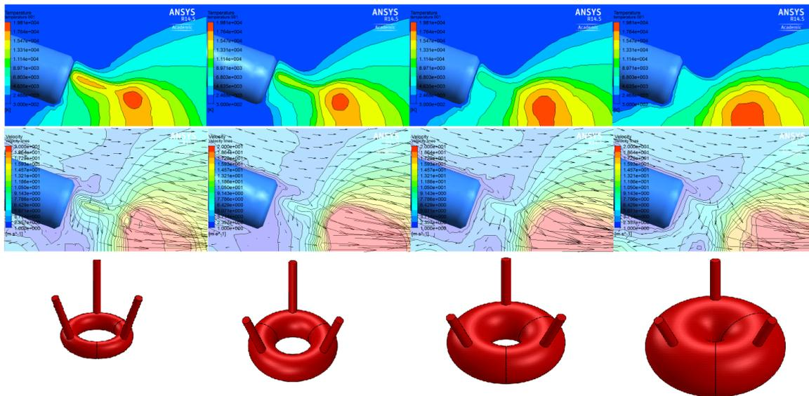
**Figure 12.** Temperature and velocity fields nearby the electrode tip (top) and arc column simplified shape (bottom) in 4 different volumes: 2 cm<sup>3</sup>, 4 cm<sup>3</sup>, 8 cm<sup>3</sup> and 16 cm<sup>3</sup>.
