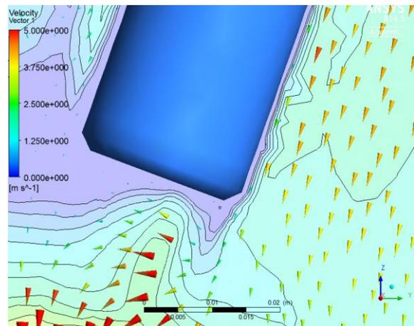
**Figure 10.** Velocity field around the electrode tip.
