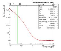
Fig. 8 – An example of the in-phase third harmonic power from a frequency sweep of a Rohacell sample.
