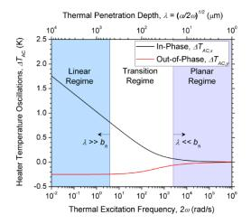
Fig. 1 – The in-phase and out-phase components of the  $3\omega$  temperature oscillations. In the low frequency limit, below the transition regime, the linear approximation may be used (taken from de Koninck, 2008).
