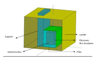
Fig. 14 – AERSUS Instrument Components
