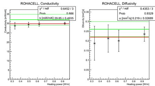
Fig. 9 – Thermal conductivity and diffusivity measurement of Rohacell performed at AST-DE.
