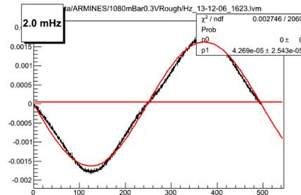
Fig. 6 – Voltage across the Wheatstone bridge removes most of the 1st harmonic as well as common mode harmonic distortion.
