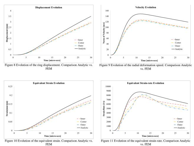
The advantage of the finite element model resides in its ability to provide us with information on the local phenomena taking place during the forming process. When looking at the strain-rate for instance (Figure 11) it is found that the inner region withstands the largest strain-rates during most of the process, but the peak is actually found for the central and outer elements. This might be due to the transmission of the shock wave through the solid domain.
