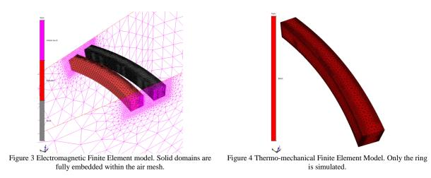
Within MATELEC we set-up all the electromagnetic properties of the study case plus the electric constants defining the machinery behind the process. Namely, the initial potential (energy level); the equivalent capacitance of the machine; and the equivalent resistance and inductance of the circuit connected from the machine to the coil. These four parameters are introduced as the driving values for the whole simulation.
