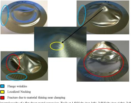
Figure 18 Experimental results of a flat sheep metal expansion. Trails at 1.5kVolts (top-left), 2.5kVolts (top-right), 2.65kVolts (bottom-left) and 3kVolts(bottom right).
