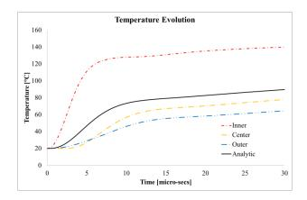
Figure 14 Evolution of the temperature increase due to self heating and joule heating. Analytic vs. FEM
