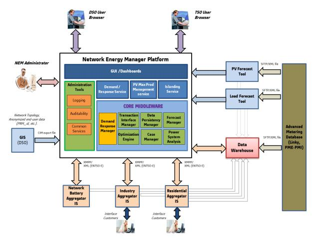
Figure 3: general architecture of the DER Management System
