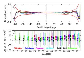
**Figure 4.** (a) Cosine response from laboratory tests. Shown error is normalized by incoming beam intensity. Thermopile readings are shown in different colours. Red envelope lines show the  $\pm 2$ % limits (from ISO 9060/1990). (b) SPN1 – TBM differences distributions for DNI, GHI and DHI as a function of bins of SZA at all stations. Box size represents the percentiles 25 and 75. Whiskers account for 99.3% of data under Gaussian distribution assumption.
