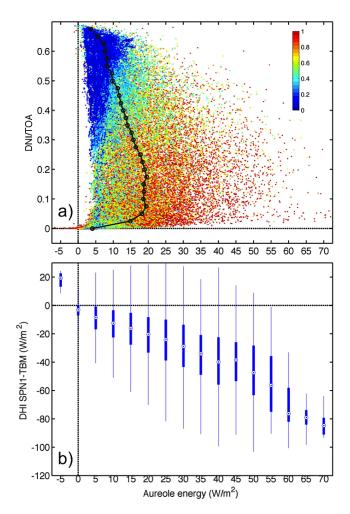
**Figure 7.** (a) DNI/TOA vs. aureole energy; colour scale corresponds to CF (CF = 0 in blue, CF = 1 in red). Black line represents the mean aureole values for each 0.025-wide bin of DNI/TOA. (b) DHI SPN1 – TBM differences in box plots as a function of aureole energy at Winster. Box sizes account for 25–75 percentile interval. Whisker length corresponds to approximately  $\pm 2.7\sigma$  and 99.3% coverage if the data are normally distributed.
