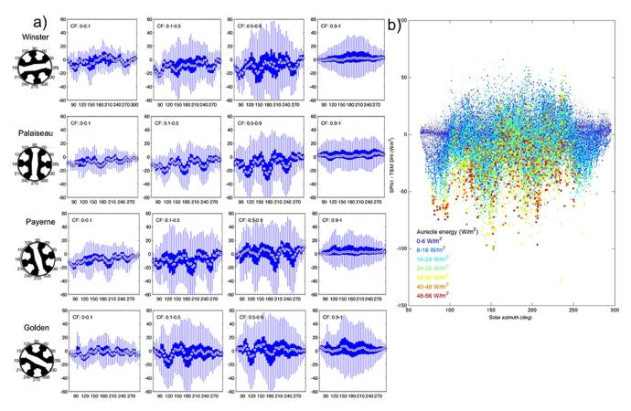
**Figure 8.** DHI differences (in W m<sup>-2</sup>) as a function of solar azimuth angle (in degrees) and for different (**a**) cloud fraction values at Winster, Palaiseau, Payerne and Golden and (**b**) aureole intensities at Winster. The SPN1 shadow mask orientation with respect to solar azimuth  $(0^{\circ} = N)$  is shown for each site (circle drawings on the left). SPN1 values have been recalibrated as described in Sect. 4.2.
