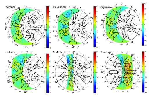
Figure 10. DHI differences (TBM – SPN1) as in Fig. 9 with the 10° first-touch-angle isolines superimposed for all sites. SPN1 values have been recalibrated as described in Sect. 4.2.
