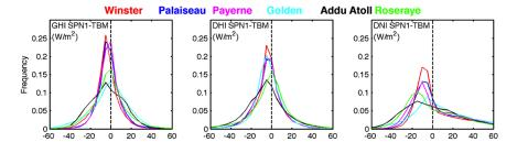
Figure 3. SPN1 – TBM difference distributions (after slope calibration) for GHI (left), DHI (centre) and DNI (right) irradiance at all sites.
