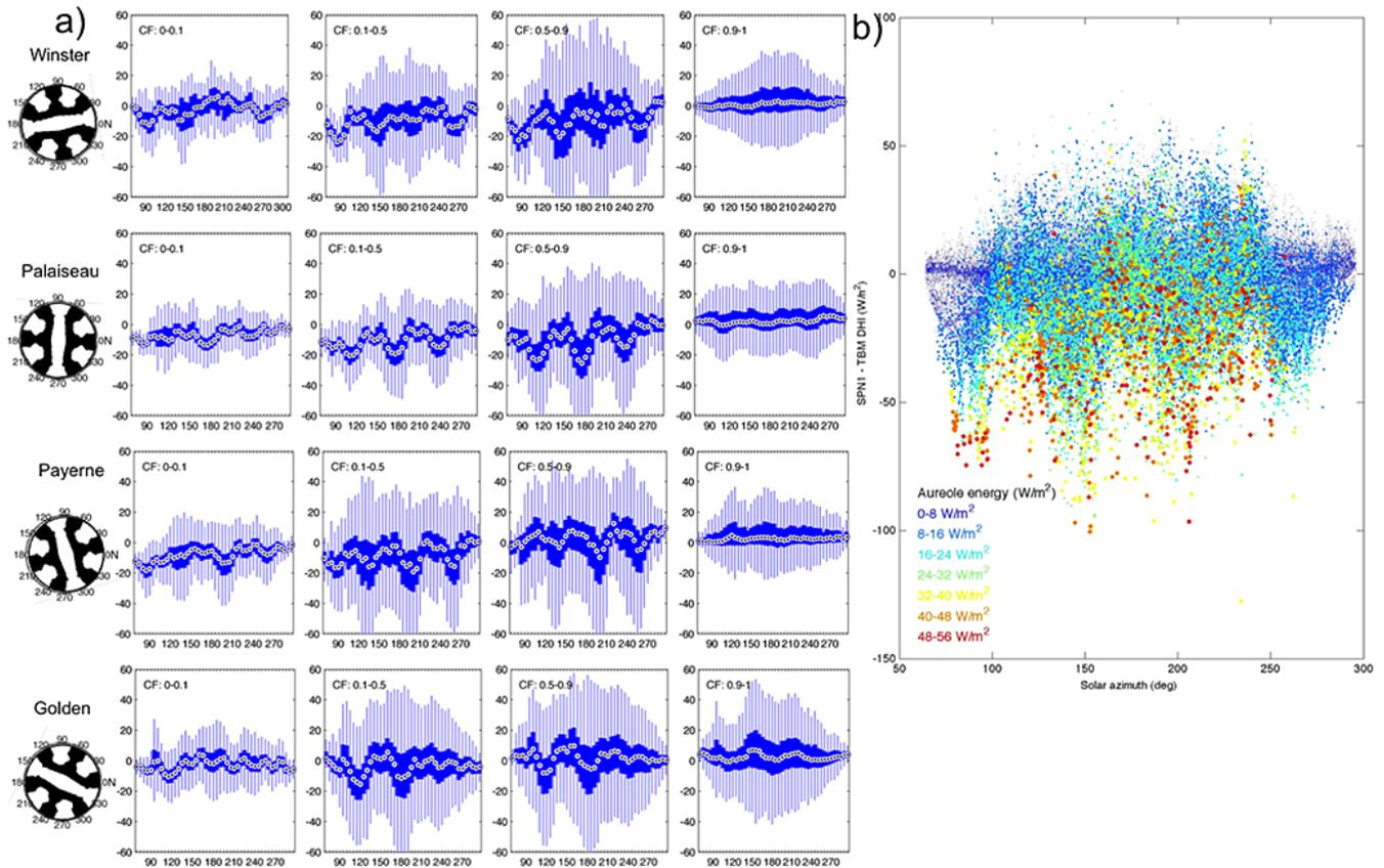
**Figure 8.** DHI differences (in  $\text{W m}^{-2}$ ) as a function of solar azimuth angle (in degrees) and for different (a) cloud fraction values at Winster, Palaiseau, Payerne and Golden and (b) aureole intensities at Winster. The SPN1 shadow mask orientation with respect to solar azimuth ( $0^\circ = N$ ) is shown for each site (circle drawings on the left). SPN1 values have been recalibrated as described in Sect. 4.2.
