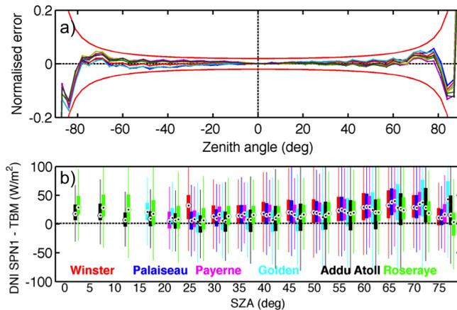
**Figure 4.** (a) Cosine response from laboratory tests. Shown error is normalized by incoming beam intensity. Thermopile readings are shown in different colours. Red envelope lines show the  $\pm 2\%$  limits (from ISO 9060/1990). (b) SPN1 – TBM differences distributions for DNI, GHI and DHI as a function of bins of SZA at all stations. Box size represents the percentiles 25 and 75. Whiskers account for 99.3 % of data under Gaussian distribution assumption.
