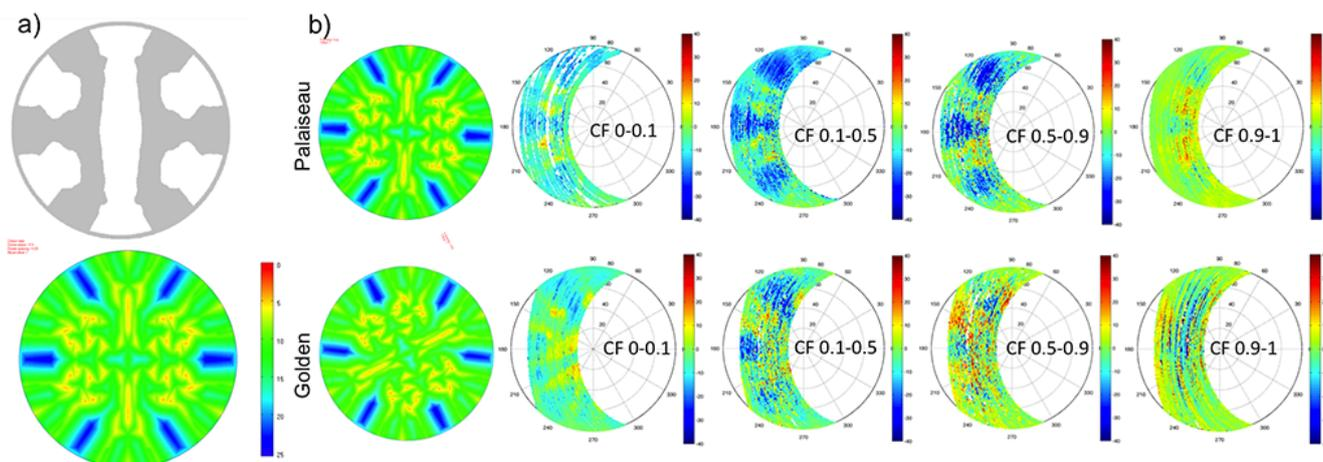
**Figure 9.** (a) Modelled diffuse first touch angles for the SPN1 relative to the shadow mask. Colour scale gives angle in degrees. (b) DHI differences (TBM – SPN1) in polar coordinates (of SZA and SAA) at Palaiseau and Golden for different bins of CF with the first touch angles pattern rotated for easier visual comparison.
