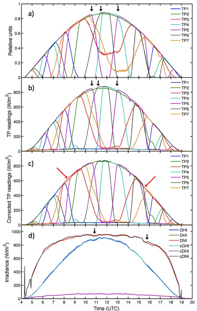
**Figure 5.** (a) Theoretical model of reading outputs from each of the SPN1 7 individual thermopiles (TPs), including dome lensing, for 1 August 2013 at Payerne. (b) Actual SPN1 TP readings for this same day and place on a clear-sky day. (c) TP readings after correction for dome lensing. (d) Measured and corrected GHI, DHI and DNI measurements for this clear-sky day.
