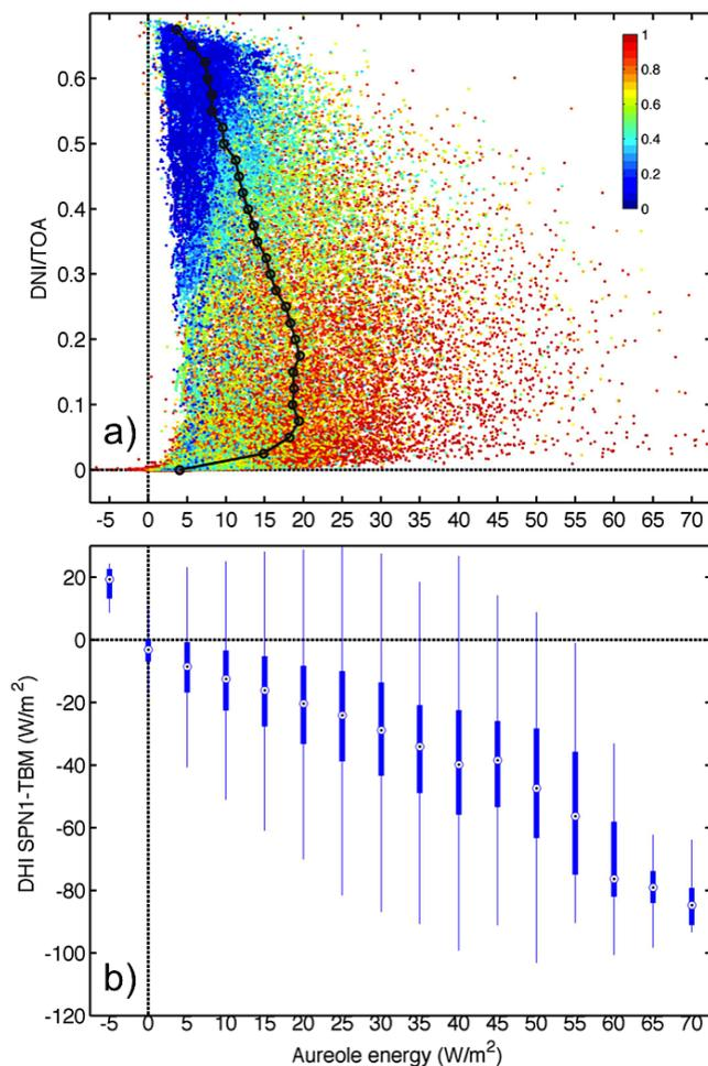
**Figure 7.** (a) DNI/TOA vs. aureole energy; colour scale corresponds to CF (CF = 0 in blue, CF = 1 in red). Black line represents the mean aureole values for each 0.025-wide bin of DNI/TOA. (b) DHI SPN1 – TBM differences in box plots as a function of aureole energy at Winstar. Box sizes account for 25–75 percentile interval. Whisker length corresponds to approximately  $\pm 2.7\sigma$  and 99.3% coverage if the data are normally distributed.
