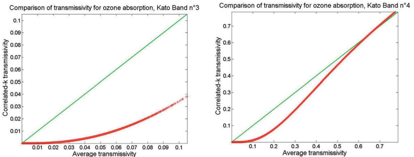
**Figure 4:** Scatterplots of transmissivity due only to ozone absorption between average by weighting with the extraterrestrial spectrum (horizontal axis) and the correlated- $k$  approximation for KB no. 3 (left) and no. 4 (right).
