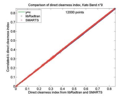
**Figure 2:** Scatterplot between spectrally detailed calculations (horizontal axis libRadtran and SMARTS) and the correlated-*k* approximation of KATO et al. (1999). Direct clearness index for KB no. 9 [518, 540] nm.
