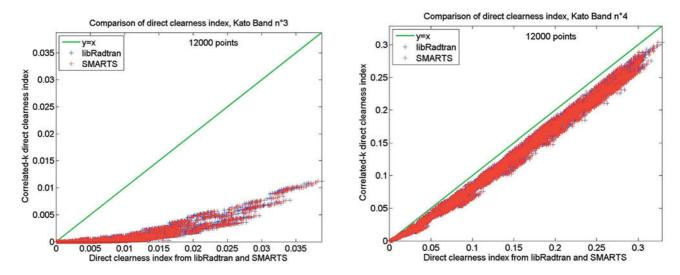
**Figure 3:** Scatterplot between spectrally detailed calculations (horizontal axis libRadtran and SMARTS) and the correlated-*k* approximation of KATO et al. (1999). Direct clearness index for KB no. 3 [283, 307] nm (left) and no. 4 [307, 328] nm (right).
