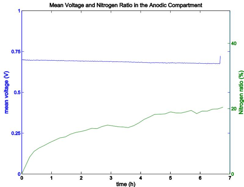
Fig : Mean Voltage and Nitrogen accumulation during a 6h45 long test of the PSR system at 0.5 A/cm<sup>2</sup>
