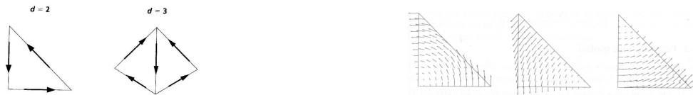
Fig. 2.a. 2D or 3D edge elements; Fig. 2.b. Edge element shape functions for 2D edge elements
