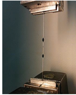
Fig. 2. Experimental device for identification of material behaviour of the strands.
