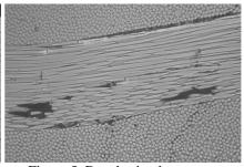
Figure 3. Debonding fiber/matrix
