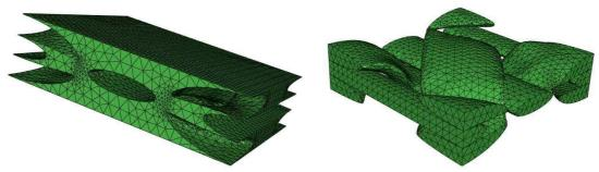
Figure 2. Periodic mesh of the unit cell
