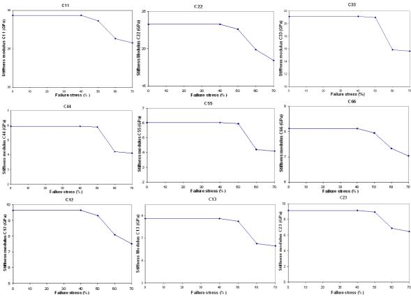
Figure 9. Evolution of stiffness coefficients according to mechanical loading in a tensile test
