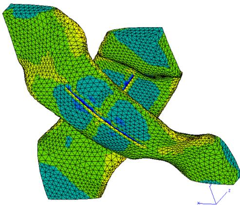
Figure 7. Introduction of a crack on off-axial yarns
