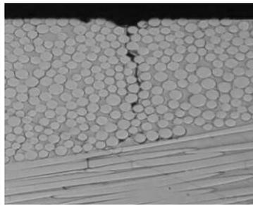
Figure 4. Transverse cracks
