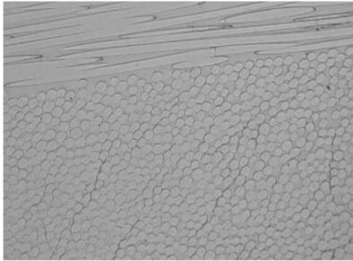
Figure 3. Debonding fiber/matrix
