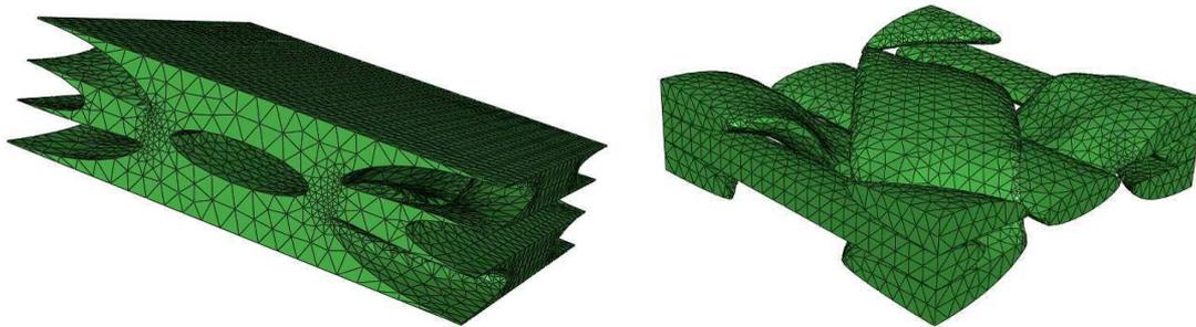
Figure 2. Periodic mesh of the unit cell
