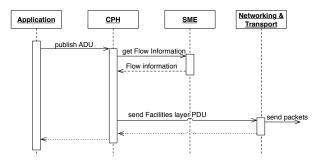
Fig. 4. Application Data Unit Transmission.
