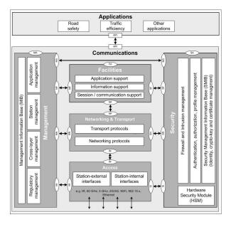
Fig. 1. ITS Station reference architecture [7].
