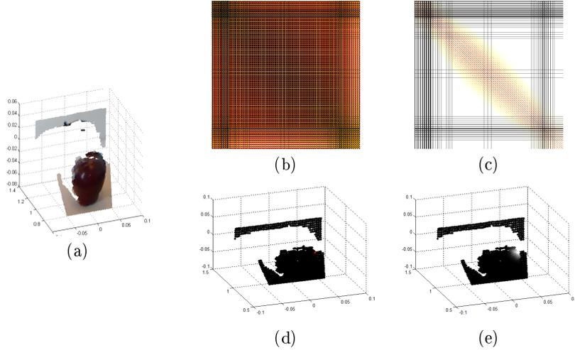
**Fig. 2.** Heat kernel at a given point: (a) RGB-valued point cloud  $f(x_i)$  of  $N$  points; (b) matrix of all-pairs of Euclidean distances  $d^{Euclid}(x_i, x_j)$ ,  $1 \leq i \leq N$ ,  $1 \leq j \leq N$ ; (c) matrix of all-pairs of heat distances  $d_T^{Heat}(x_i, x_j)$ ,  $1 \leq i \leq N$ ,  $1 \leq j \leq N$ ; (d) in red, a given point  $x_k$ , (e) heat kernel  $p_t(x_k, x_i)$  at this point  $x_k$ .
