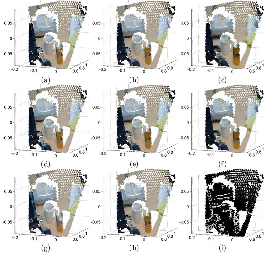
**Fig. 3.** Morphological processing a RGB-valued point cloud: (a) original image  $f(x_i)$ . Erosion  $\varepsilon_{b_t}(f)(x_i)$  with (b)  $t = 1$ ,  $T = 0.05$ , (c)  $t = 1$ ,  $T = 0.4$ , (d)  $t = 0.5$ ,  $T = 0.1$ , (e)  $t = 1$ ,  $T = 0.1$ , (f)  $t = 2$ ,  $T = 0.1$ . (g) Dilation  $\delta_{b_t}(f)(x_i)$  with  $t = 1$ ,  $T = 0.1$ . (h) opening  $\gamma_{b_t}(f)(x_i)$  and (i) top-hat transform  $f(x_i) - \gamma_{b_t}(f)(x_i)$  with  $t = 1$ ,  $T = 0.1$ .
