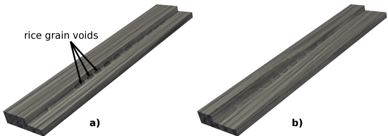
Figure 3. X-ray tomography images. (a) Initial microstructure with voids; (b) Microstructure after deformation: void growth.
