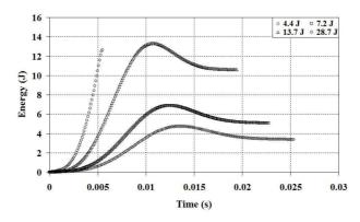
**Figure 3.** Energy-Time histories for different impact energy levels.
