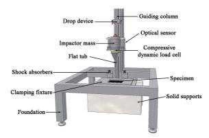
**Figure 1.** Schematic diagram of drop-weight impact testing machine.
