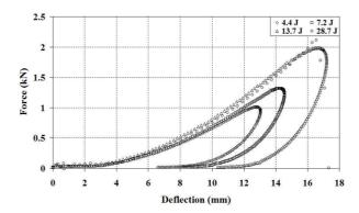
Figure 2. Force-Deflection diagrams for different impact energy levels.
