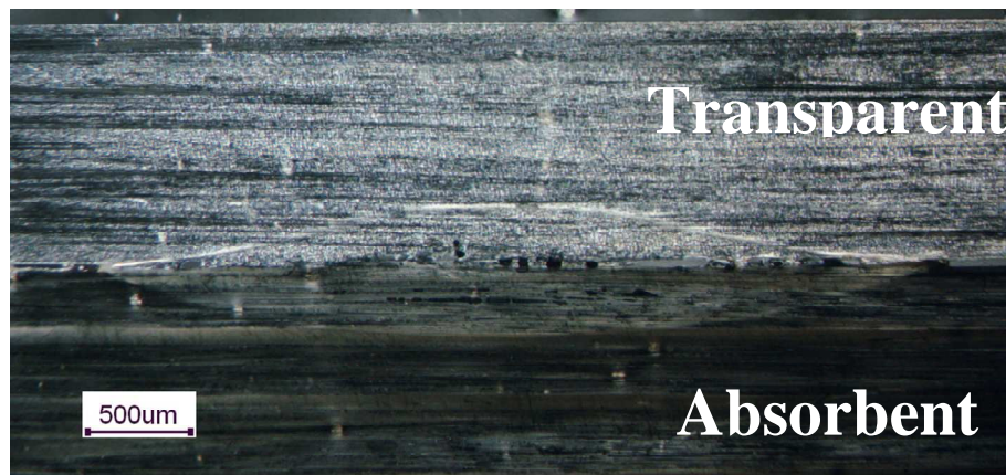
Figure 2. The laser weld seam geometry obtain after microtome cuts [8].
