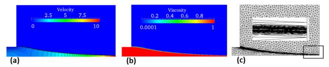
FIGURE 4. (a) Velocity profile, (b) The viscosity distribution, (c) The obtained mesh
