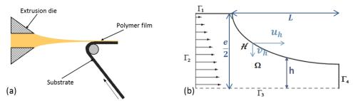
FIGURE 1. (a) Schematic of the coating process, (b) Half flow domain of fluid
