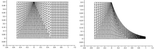
FIGURE 2. Structured mesh transformation
