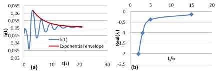
**FIGURE 5**. (a) Transient stability analysis, (b) Leading eigenvalue evolution as a function of  $\frac{L}{e}$
