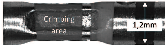
Fig. 9. Contact shape after crimping.
