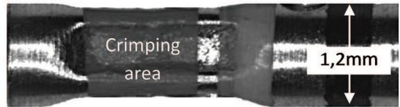
Fig. 9. Contact shape after crimping.
