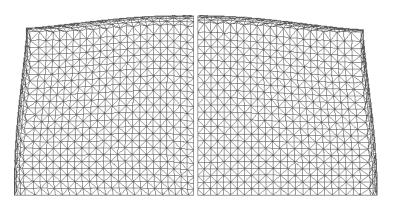
**Figure 7.** *Upper view of the intermediate block with multi-bodies calculation (left) and with single body calculation (right)*
