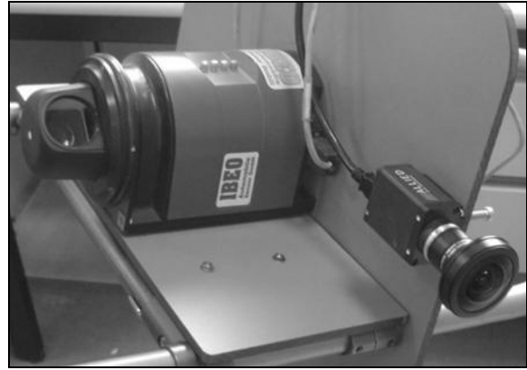
Figure 6 Plate-forme rigide scanner laser/caméra
