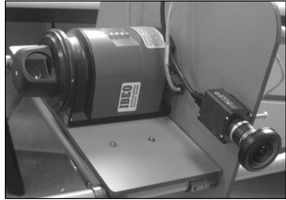
Figure 6 Plate-forme rigide scanner laser/caméra
