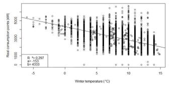
Fig.11. Thermo-sensitivity of the measured load curve of Fig. 10 where the temperature is the temperature of the cities of the customers weighted with the number of customers in the cities.
