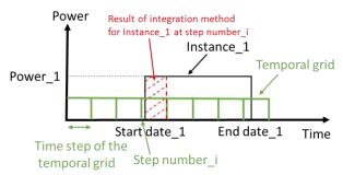
Fig.4. Illustration of the way the evaluation of energy is done in the simulator
