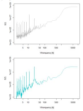
Fig.7. Spectrum of a load curve of a medium voltage feeder (upper grey curve) and the simulated load curve (lower turquoise curve), for a whole year.
