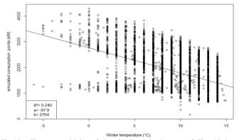
Fig.12. Thermo-sensitivity of the simulated load curve of Fig. 10 by taking a medium level of thermal resistance per buildings, where the temperature is the temperature of the cities of the customers weighted with the number of customers in the cities.
