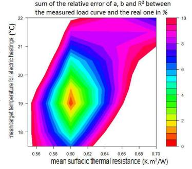
Fig.13. Sum of the relative errors between a, b and R<sup>2</sup> from simulated outputs of simulator and from the measurements, as a function of the surface thermal resistance and the target temperature.
