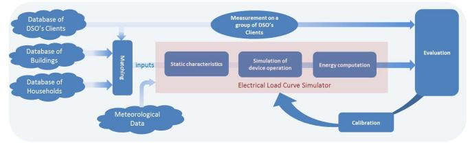
Fig.1. Illustration of the approach used for electric load curve simulation
