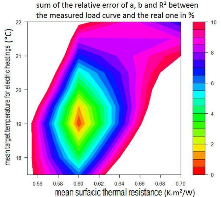
Fig.13. Sum of the relative errors between  $a$ ,  $b$  and  $R^2$  from simulated outputs of simulator and from the measurements, as a function of the surface thermal resistance and the target temperature.
