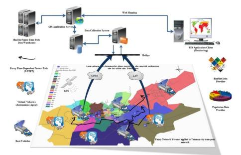
**Figure 1.** An Intelligent Transport System that includes DGT fleet monitoring, Data Collection, Virtual vehicles injection, GIS application, Database, Route planning considering travel-time and risk on a Fuzzy Voronoi Graph transport network
