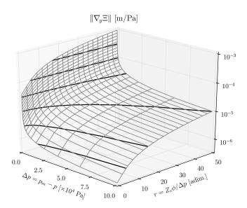
Figure 3: Sound to lip height sensitivity, with iso-value curves in black.
