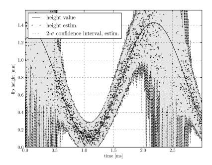
Figure 1: Lip height estimation and standard deviation
