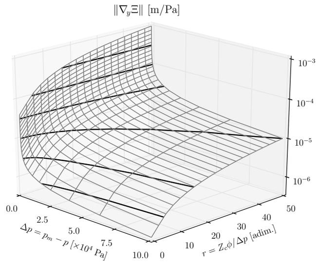
Figure 3: Sound to lip height sensitivity, with iso-value curves in black.
