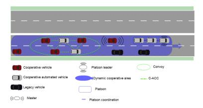
Figure 2. Motorway illustration of a *local cooperative area*. Since vehicles are moving at a very similar speed, there is a clear benefit to have a moving area,
