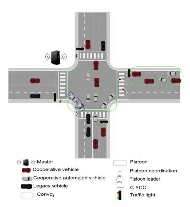
Figure 4. Urban case: the whole intersection is a *local cooperative area*. Here the infrastructure organizes the cooperation so that we have a *static cooperative area*. The *convoy* structure can be used to synchronize vehicles (or *platoons*) passing by the intersection.
