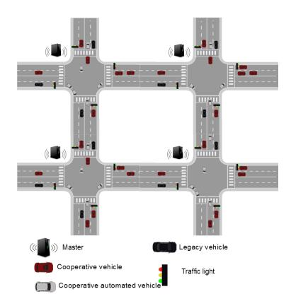
Figure 5. As in the motorway case, traffic management takes benefit of a grouping of *local cooperative areas* into a *global cooperative area* in order to build a more comprehensive scheme.
