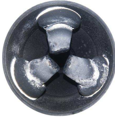
Figure 1: Top view of the discharge zone, the three electrodes are in planar position.
