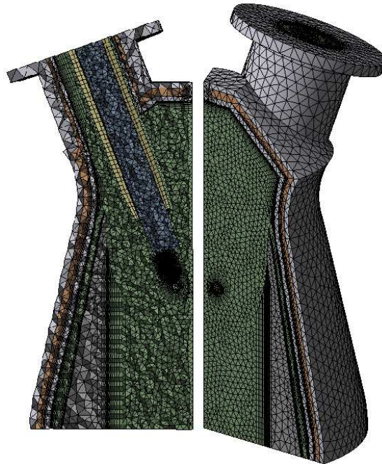
Figure 3: Meshing of the simplified geometry (right: cross section in the middle plane, left: exterior meshing)
