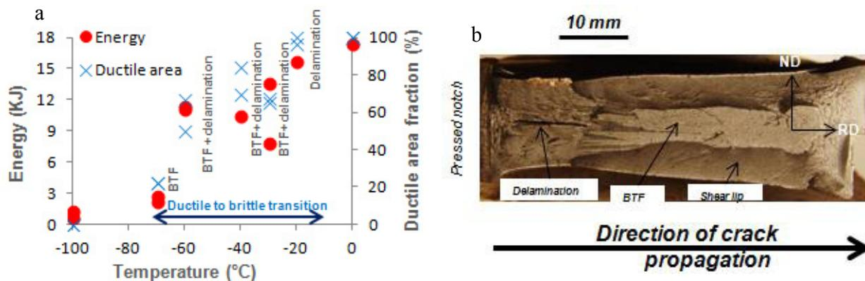
Fig. 1. (a) BDWTT behavior (loading along TD, crack propagation along RD); (b) Fracture surface ( $T = -40^\circ\text{C}$ ).
