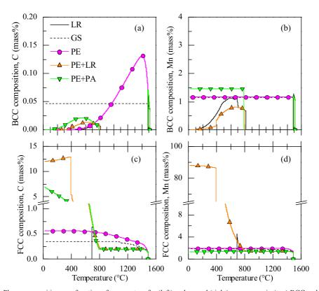
**Fig. 6.** Phase composition as a function of temperature for (left) carbon and (right) manganese in (top) BCC and (bottom) FCC phases. Steel S-2 (Table 1), 5 microsegregation models. (Online version in color.)
