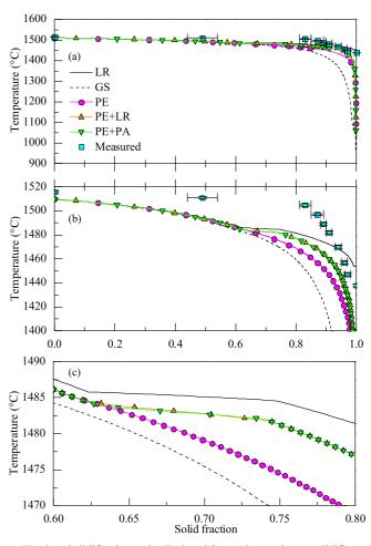
Fig. 2. Solidification paths displayed for (a) the maximum solidification interval deduced from the predictions, (b) the experimental range, and (c) around the peritectic reaction. Measurement data are added for comparison. Steel S-1 (Table 1), 5 microsegregation models. (Online version in color.)
