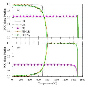
Fig. 4. Mass fraction of phases as a function of temperature for (top) δ-BCC and (bottom) γ-FCC. Steel S-2 (Table 1), 5 microsegregation models. (Online version in color.)
