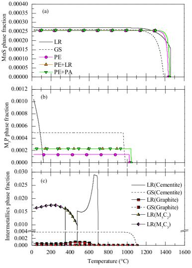
Fig. 5. Mass fraction of phases as a function of temperature for (top) MnS, (middle) M<sub>3</sub>P and (bottom) other intermetallics. Steel S-2 (Table 1), 5 microsegregation models. (Online version in color.)
