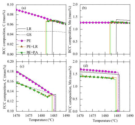
Fig. 3. Phase composition within the temperature range of the peritectic transformation for (left) carbon and (right) manganese in (top) BCC and (bottom) FCC phases. Steel S-1 (Table 1), 5 microsegregation models. (Online version in color.)
