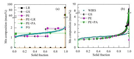
Fig. 7. Average Mn composition as a function of the mass fraction of solid with (left) FG and (right) WIRS sorting methods. Steel S-2 (Table 1), 5 microsegregation models. Parameters for the WIRS analysis are given in Table 3. (Online version in color.)
