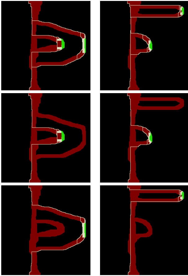
Fig. 15. Reconnections of the disconnected components in green into the loops to the top and bottom faces. 2D vertical 4-connectivity reconstructions along Oy .
