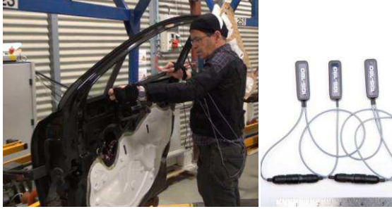
Figure 2 : On the left, a worker fitting the windows sealing-sheet on a door in the experimental cell of PSA, while he wears the AnimaZoo™ IGS120+; on the right 3 inertial sensors from IGS120+.
