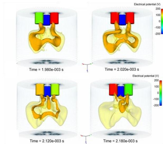
**Fig.4** Arc shapes obtained with the MHD modeling, displayed on a front view by a 8 000 K isosurface temperature and the hot channels are displayed by a 5 000 K isosurface temperature. Electrodes are colored by the electrical potential value.
