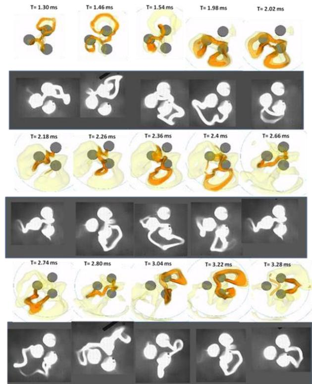
**Fig.3** Comparison of the arc shapes, displayed by a 10 000 K isosurface temperature and hot channels displayed by a 5 000 K isosurface temperature, with the arc video sequence by a bottom view of the inter electrode gap.
