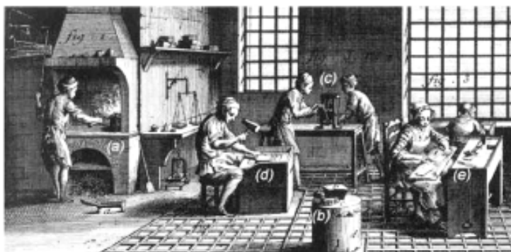
Fig. 9. A goldbeater workshop at 18 th century [from 20]; (a) ingot melting; (b) cooling ingot; (c) rolling; (d) beating; (e) mould emptying and booklet packing
