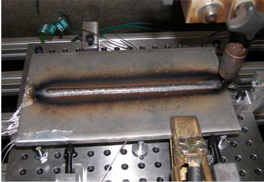
Figure 2: GMA welding experiment.
