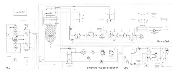
Figure 1. Simplified PFD of the reference oxy-combustion power plant
