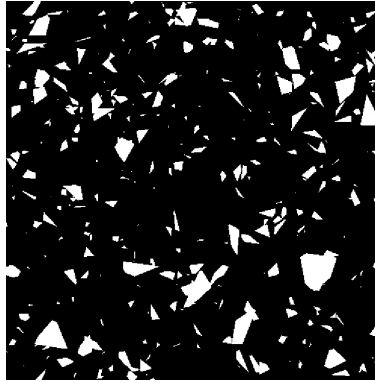
Fig. 19. 2D slice of a 3D Boolean Poisson polyhedra realization
