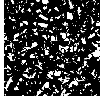
Figure 6: 2D cut of a Boolean Poisson polyhedra model of size 500^3 with \lambda=0.045 and p=0.2 .
