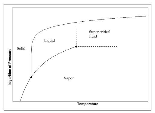
Fig. 1. Pure compound Pressure-Temperature phase diagram. ( $\blacktriangle$ ) Triple point, ( $\bullet$ ) : critical point. Lines : Coexistence curves
