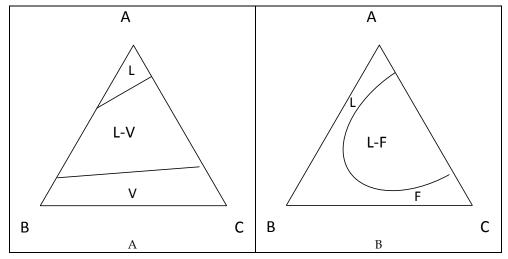
A: Vapor-Liquid Equilibria (VLE), B: if T or P is increased a supercrital fluid (F) appears and so a FLE.
