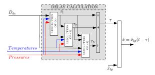
Fig. 4. Scheme of the proposed delay calculation strategy for intake burned gas fraction estimate x. The numerical solving of implicit integral equations (4)-(6) can be obtained by sampling and calculating the integrals at increasing values of  $\tau_i$  starting from 0, which are real-time compliant calculations.
