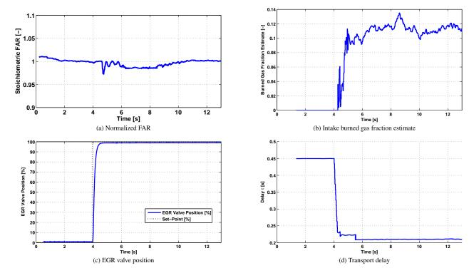
Fig. 7. Experimental results for constant engine speed ( $N_e = 2000 \text{ rpm}$ ) and transient torque request (step from IMEP = 6 bar to 12.5 bar), resulting into a delay variation. The normalized FAR response pictured in (a) uses the intake burned gas fraction estimation pictured in (b), obtained with the on-line estimation of the delay (d).
