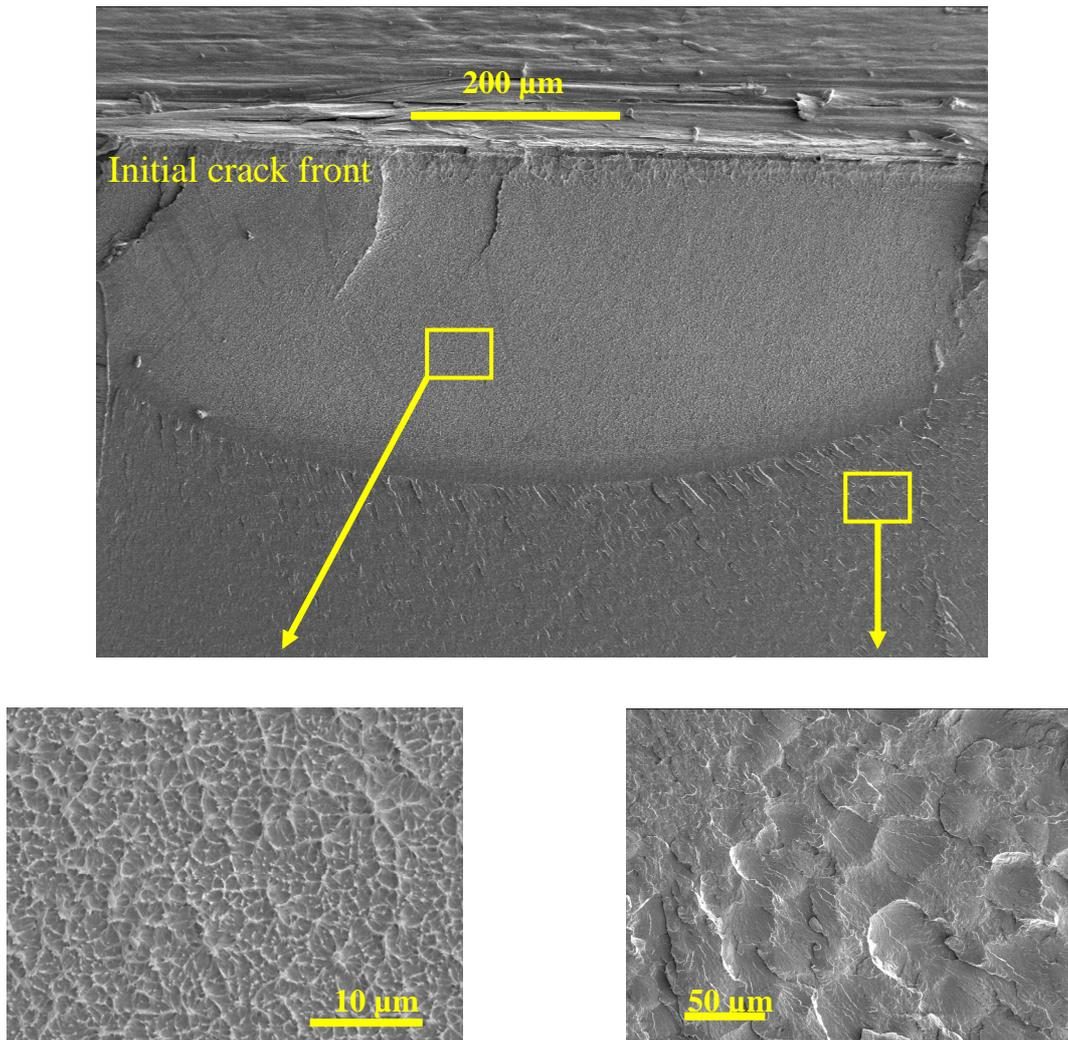
Figure 1. Typical features of semi-crystalline fracture surfaces for  $50 \leq \%F \leq 80$
